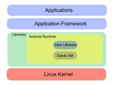
Figure 1. Android Structure
