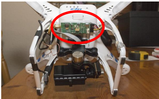
Figure 4.1 wireless video transmitter position. Wireless transmitter can be placed anywhere at the bottom of the DJI Phantom 2, and in this case mounted on the bottom of battery power.
