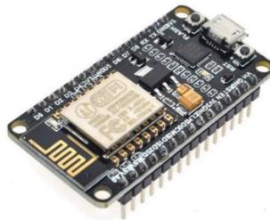
**Gambar 1** NodeMCU ESP8266[7]
