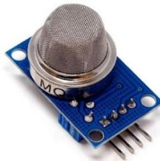
**Gambar 2** Sensor Gas MQ2[11]
